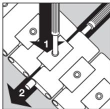
Open the push-button release safety clasp by pressing the button on the side. Lay the bracelet with its top surface on a firm base. Using the special tools provided, you can now push down the securing pin (1) at the desired point of separation and, at the same time, displace the pivot pin laterally by about 3 mm (2) with the second special tool.
