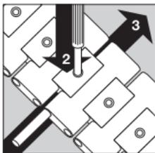
Using the special tool provided, now press the securing pin downwards (2) and, at the same time, slide the pivot pin back into the bracelet until it lies flush (3).
