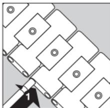
Attach the component parts of the bracelet link to the connection point, and push the pivot pin into the bracelet from the side (1).
