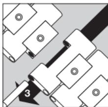
Now pull the protruding pivot pin from the bracelet (3). The metal bracelet is now separated, and you can adjust the length of the bracelet by removing or adding individual links.
